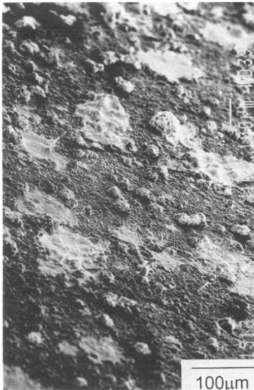
Fig. 7 Effect of spray distance on tungsten splat morphology at a plasma power of 40 kW and a chamber pressure of 200 torr. (a) Zt = 200 mm. (b) Zt = 300 mm.
